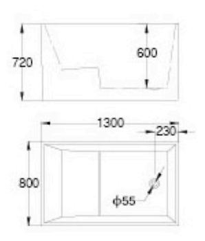
Kheub Bathroom Ware must be installed in accordance with the provisions of AS/NZS 3500 and any relevant local regulations. Installations not complying with AS/NZS 3500 may void the product and performance warranty provisions.
